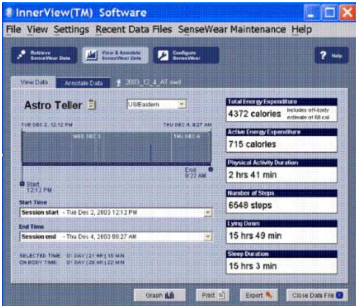
Fig. 4. InnerView™ wearer software data visualization. configure the sampling rates and duration of the 41 data collection channels on the armband. Each armband can be personalized to an individual user according to his needs for more accurate readings or longer recordings. Saved data can be exported for easy data analysis.
