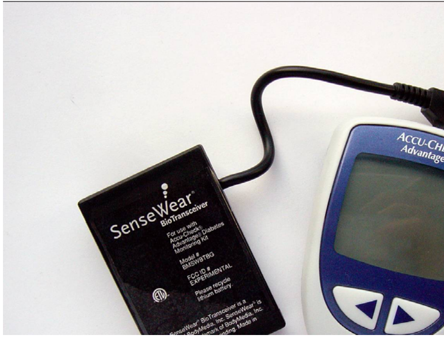
Figure 3. The SenseWear BioTransceiver that allows medical devices to communicate with the armband.
