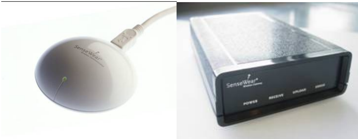
Figure 4. The SenseWear Wireless Communicator (left) and Wireless Gateway (right) allow communication with a PC or a web-server.
