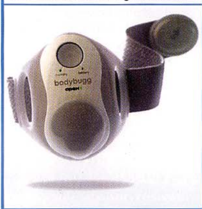
Figure 1: Armband that collects lower-level sensor readings 32 times/s.
